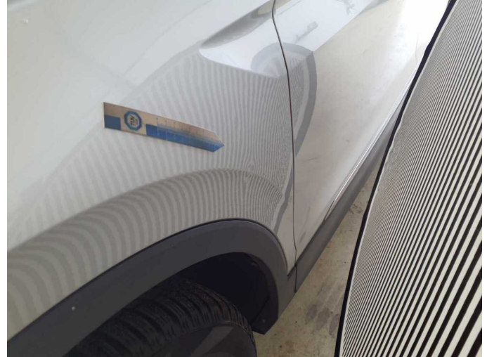
Damage 3: Mudguard - left side: Mudguard - left side - dent(s) - Repair and paint
