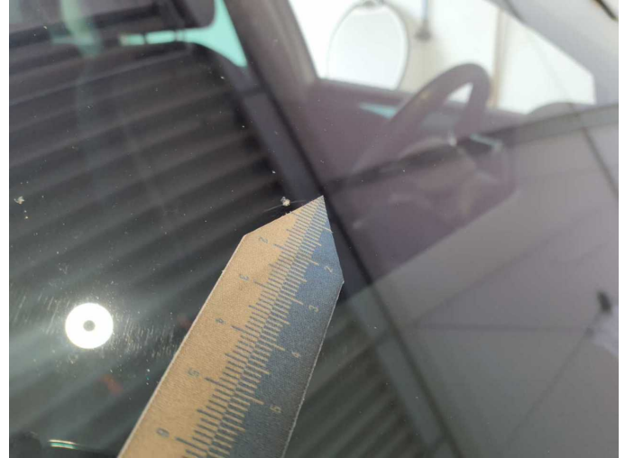
Damage 6: Vehicle glazing: Windscreen with lane departure assistant - Stone chips - Replace
