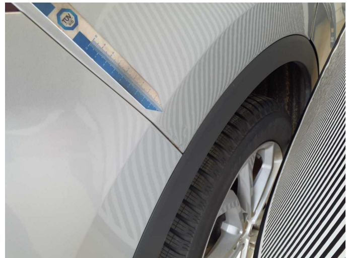
Damage 5: Side panel - rear right side: Side panel (Wellig, reißt auf. 2,5mm Spachtelschicht) - Unprofessionally repaired - Repair and paint
