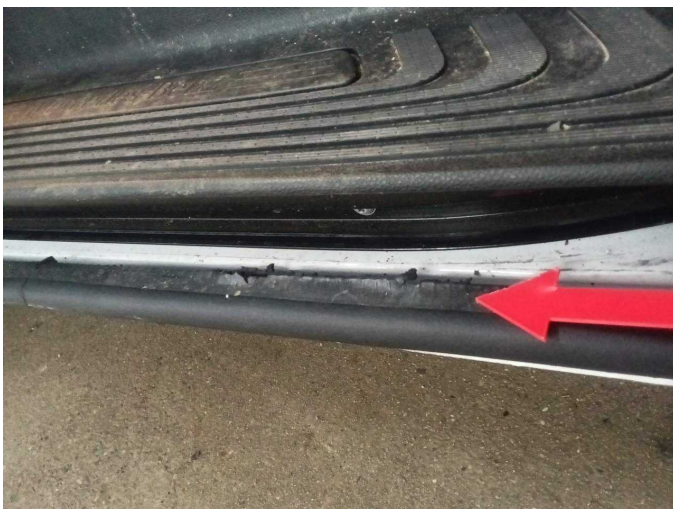
Damage 4: Sliding door, right: Door seal - Broken / torn - Replace
