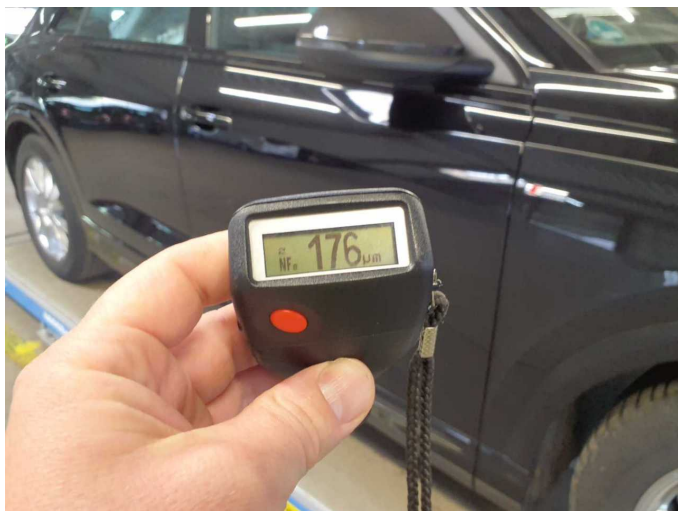
Repainting 2: Door - front right side
