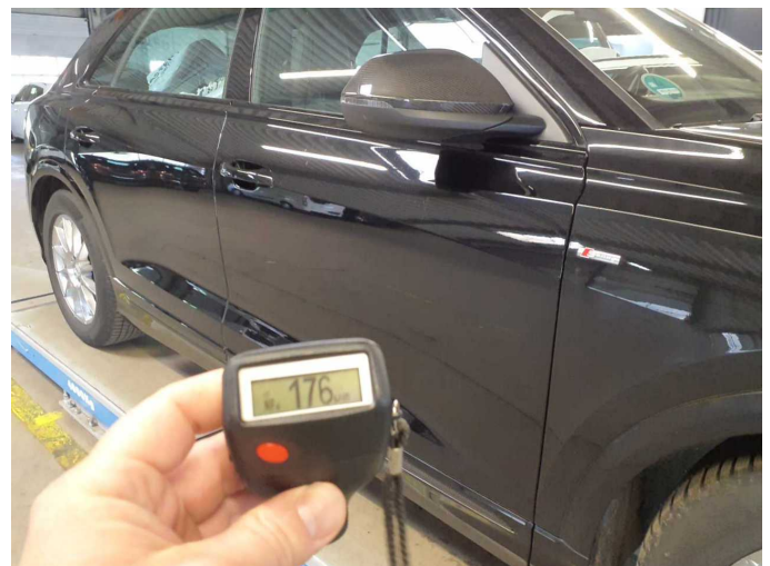
Repainting 2: Door - front right side
