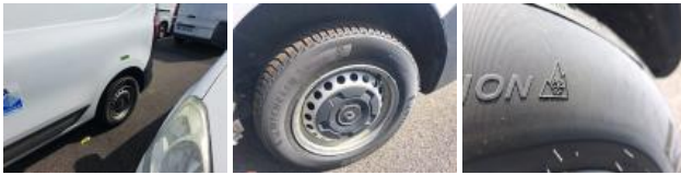
Tyre RR, Out of tolerance, Replace
