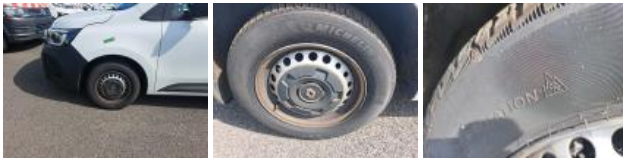
Tyre RL, Out of tolerance, Replace
