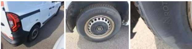
Tyre FR, Out of tolerance, Replace
