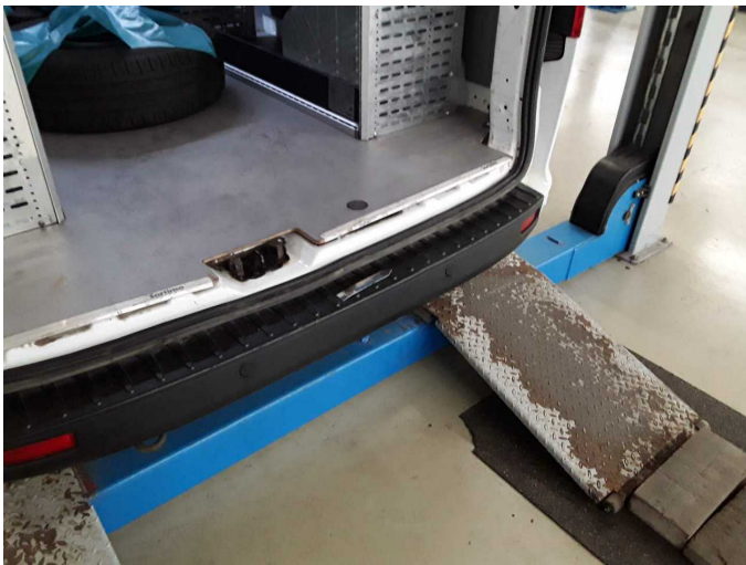
Damage 8: Rear bumper: Bumper - rear centre - Deformed - Replace
