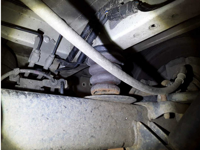
Damage 9: Rear axle: Leaf spring - right side (Anschlagpuffer links und rechts) - Porous / cracked - Replace
