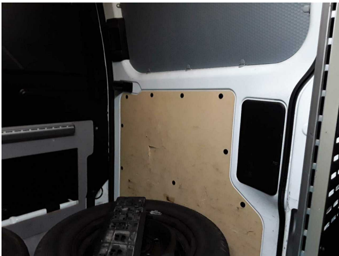
Damage 5: Sliding door, right: Trim plywood - lower - Broken / torn - Replace
