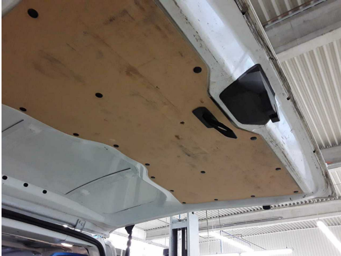
Damage 7: Boot lid / rear door: Trim rear door - plywood - lower - Broken / torn - Replace
