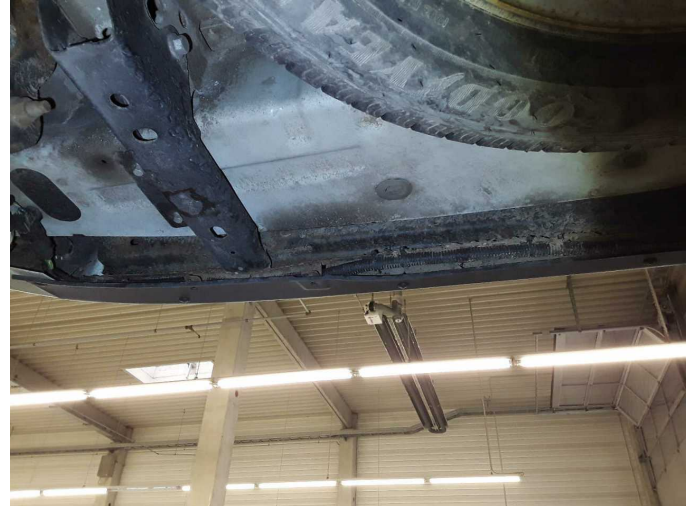
Damage 10: Rear bumper: Support - Deformed - Replace
