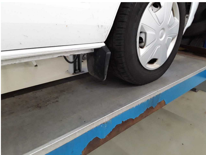
Damage 3: Mudguard - right side: Mud flap - Broken / torn - Replace
