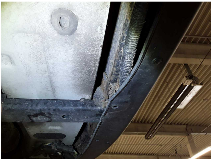
Damage 10: Rear bumper: Support - Deformed - Replace
