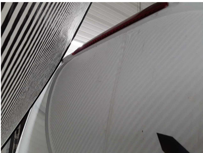
Damage 11: Boot lid / rear door: Boot lid - Dent / paintcoat damage - Repair and paint
