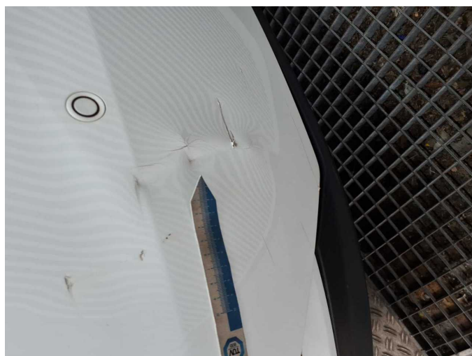
Damage 5: Rear bumper: Rear bumper - Broken / torn - Replace
