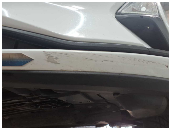
Damage 4: Front bumper: Front bumper - Scratched - Paint
