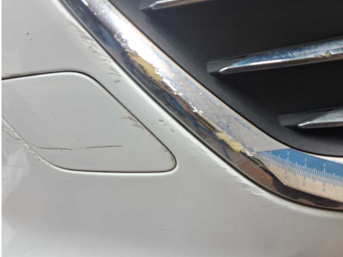
Damage 1: Bonnet: Radiator grille - Scratched - Loss in value
