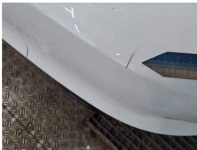
Damage 5: Rear bumper: Rear bumper - Broken / torn - Replace
