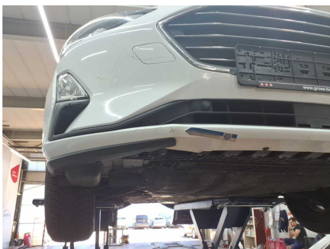
Damage 4: Front bumper: Front bumper - Scratched - Paint
