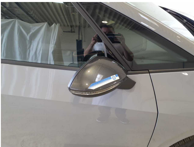
Damage 2: Wing mirror - right side: Cap - Scratched - Paint
