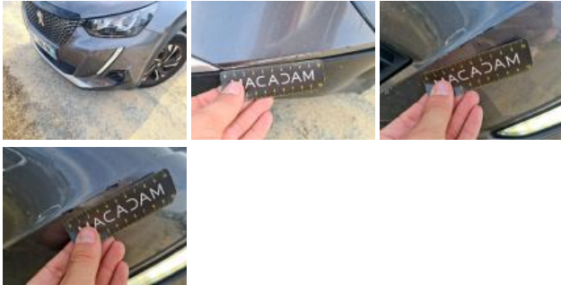
Bumper spoiler F, Deformed / Strained, Replace
