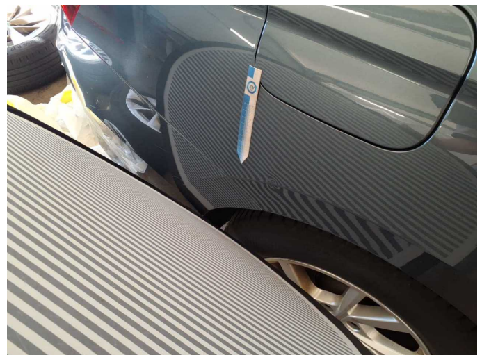
Damage 8: Side panel - rear right side: Side panel - Dent / paintcoat damage - Repair and paint
