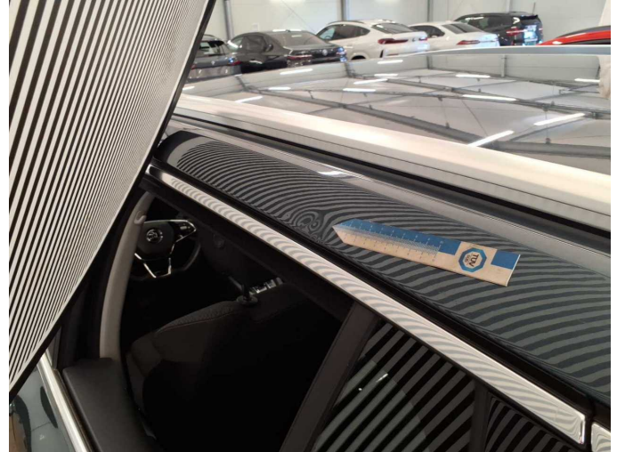
Damage 4: Roof: Roof rail - left side - dent(s) - Smooth repair work
