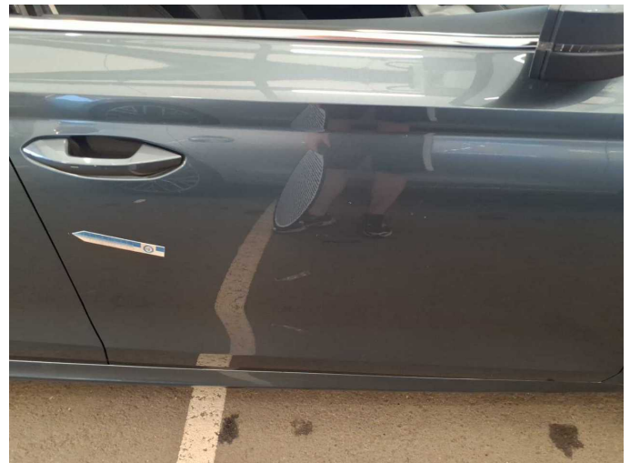
Damage 7: Door - front right side: Door - Scratch(es) - Paint
