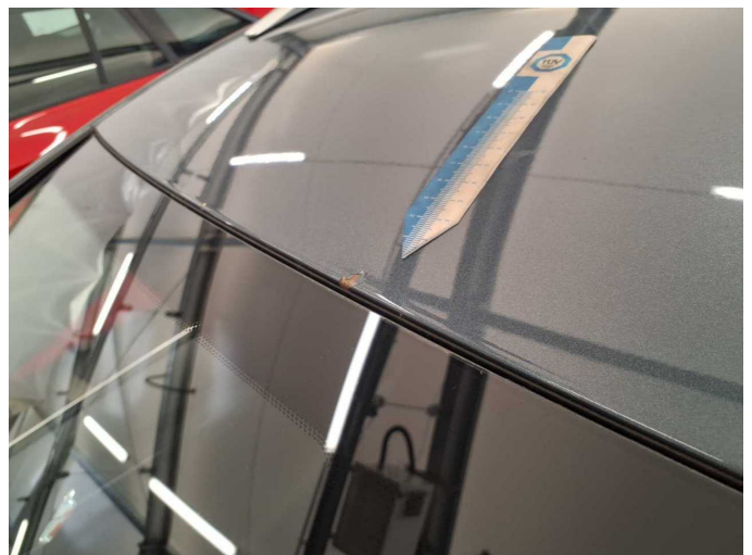
Damage 10: Roof: Roof - Corrosion - Repair and paint
