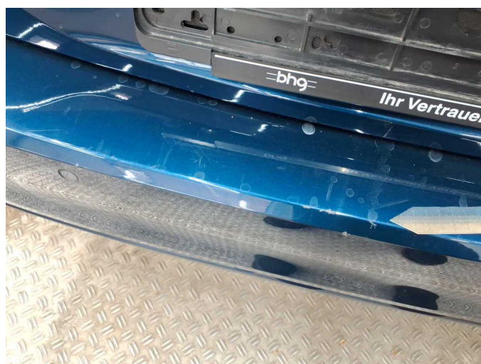
Damage 2: Rear bumper: Rear bumper - Scratch(es) - Paint
