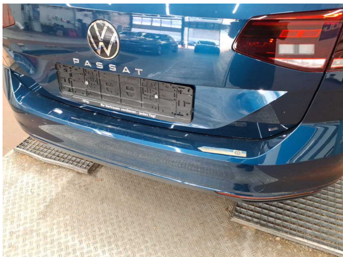
Damage 2: Rear bumper: Rear bumper - Scratch(es) - Paint
