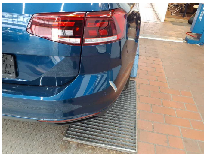
Damage 2: Rear bumper: Rear bumper - Scratch(es) - Paint
