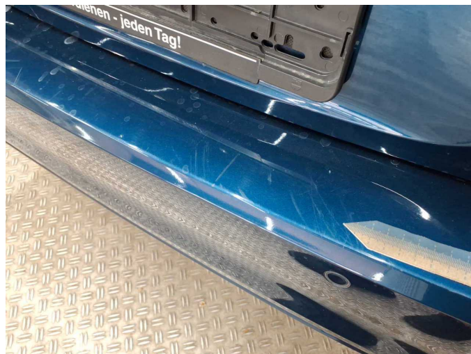
Damage 2: Rear bumper: Rear bumper - Scratch(es) - Paint
