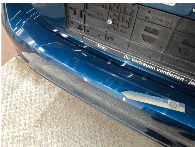
Damage 2: Rear bumper: Rear bumper - Scratch(es) - Paint
