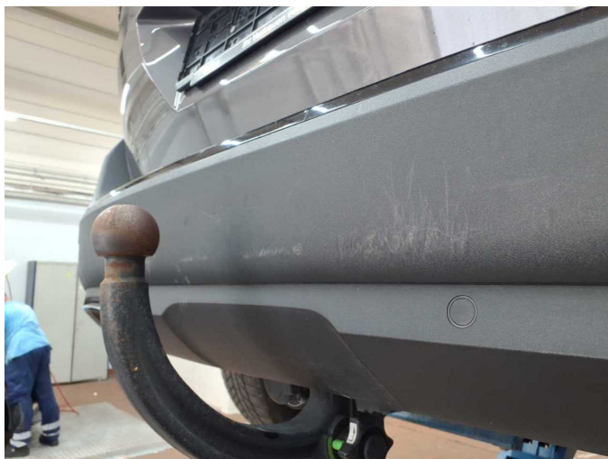
Damage 2: Rear bumper: Rear bumper (unpainted) - Scratched - Loss in value
