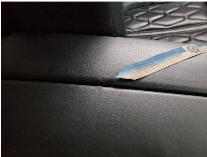
Damage 8: Interior: Interior - Scratched - Loss in value
