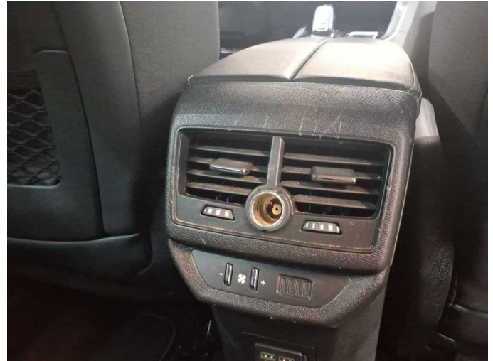
Damage 1: Electrical system: Power socket (hinten) - Incomplete - Replace
