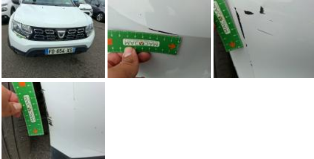
Bumper F, Broken, Replace
