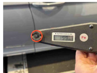
Paint thickness Door FR
