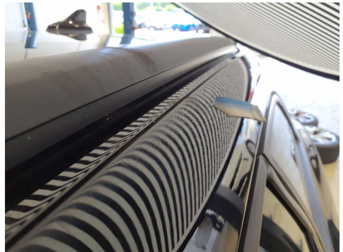
Damage 7: Roof: Roof rail - left side (Orangenhaut) - Unprofessionally repaired - Repair and paint
