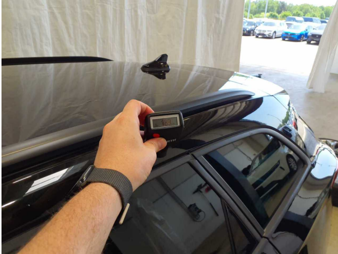
Repainting 3: Roof rail - left side
