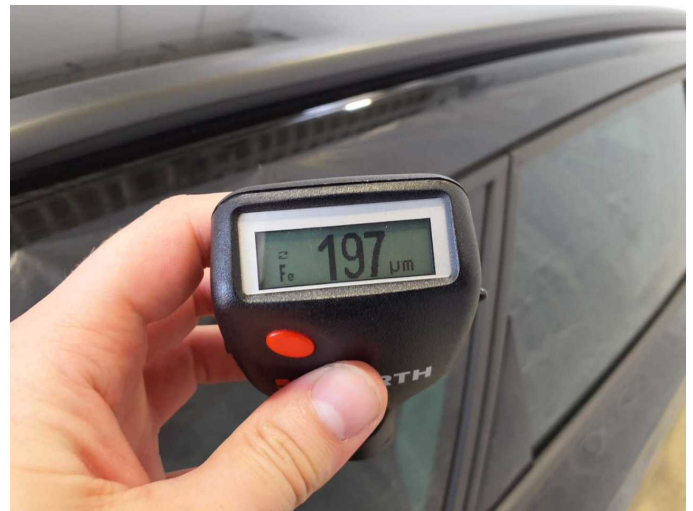
Repainting 4: Roof rail - right side
