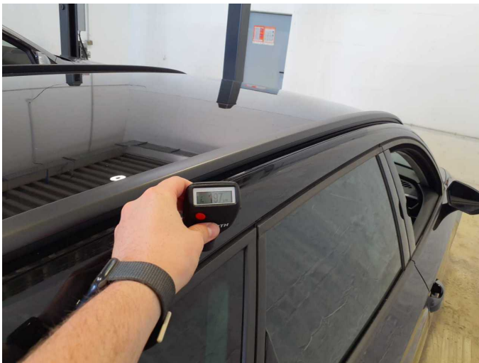
Repainting 4: Roof rail - right side
