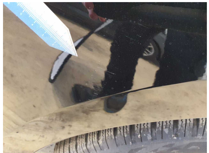
Damage 9: Mudguard - right side: Mudguard - right side - Dent / paintcoat damage - Repair and paint
