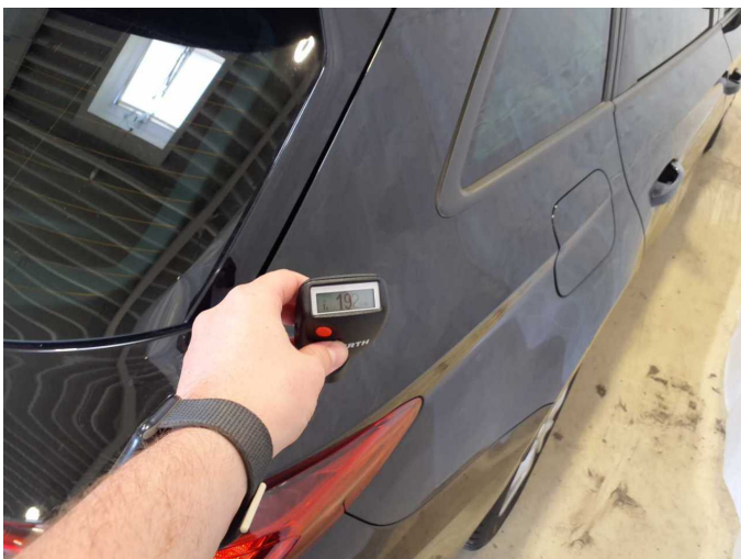
Repainting 2: Side panel - rear right side
