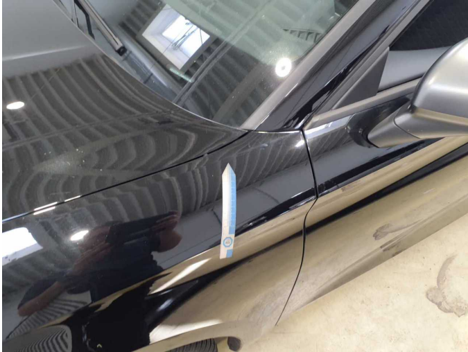
Damage 3: Mudguard - left side: Mudguard - left side (Lacknebel) - Paint defect - Conditioning
