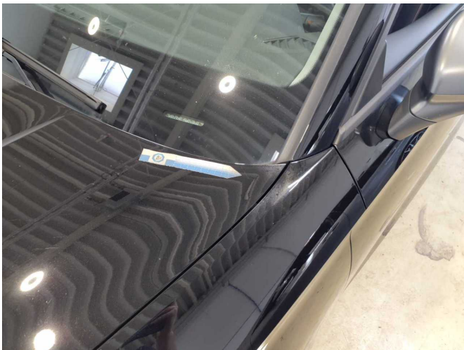
Damage 4: Bonnet: Bonnet (Lacknebel) - Paint defect - Conditioning
