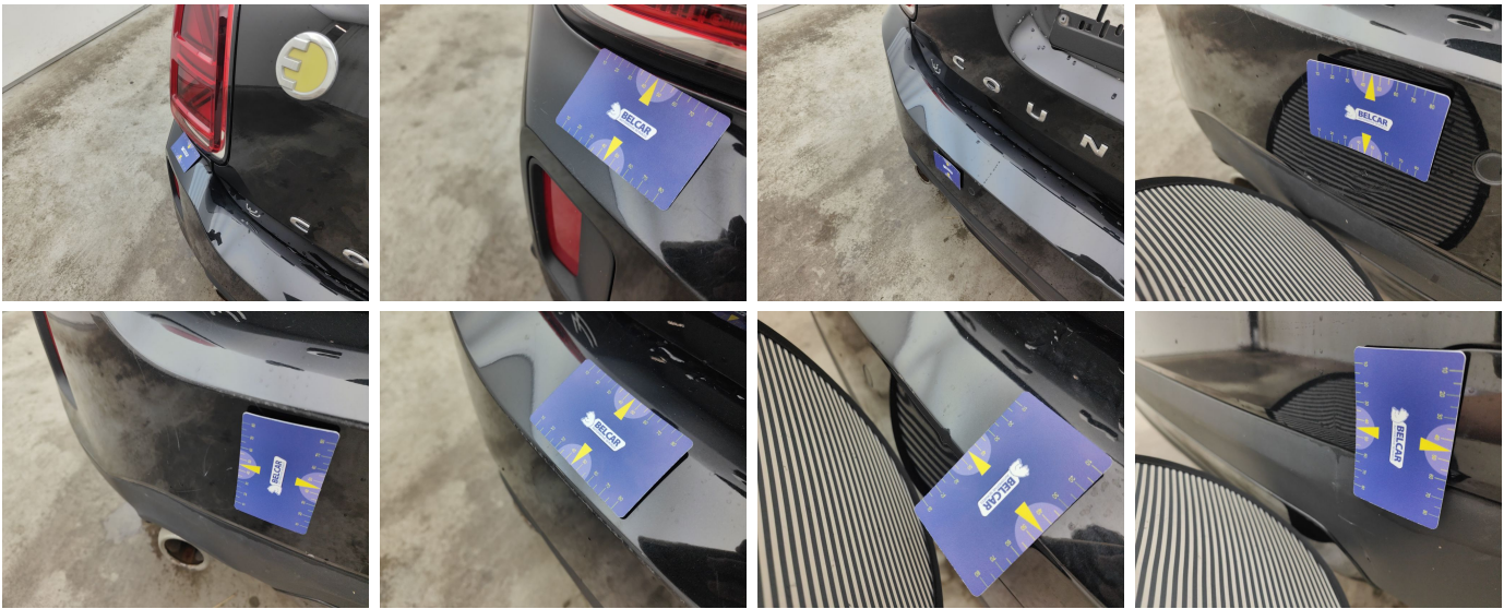
Bumper Rear // Repair & Painting-scratch + dent
