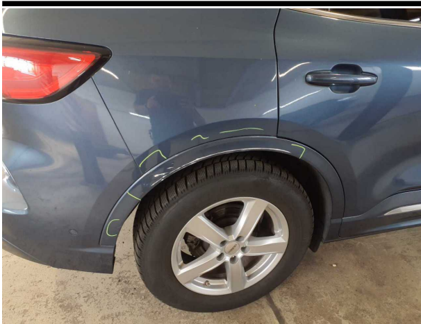
Damage #7: Side panel - rear right side: Wheel well extension - Scratched - Smart repair
