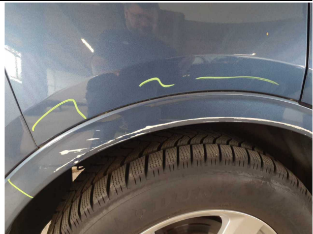
Damage #7: Side panel - rear right side: Wheel well extension - Scratched - Smart repair
