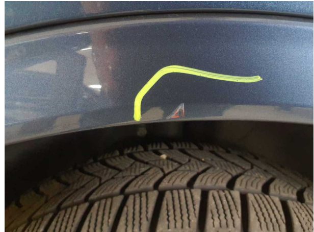
Damage #1: Mudguard - right side: Wheel well extension - Abrasion - Cover / polish
