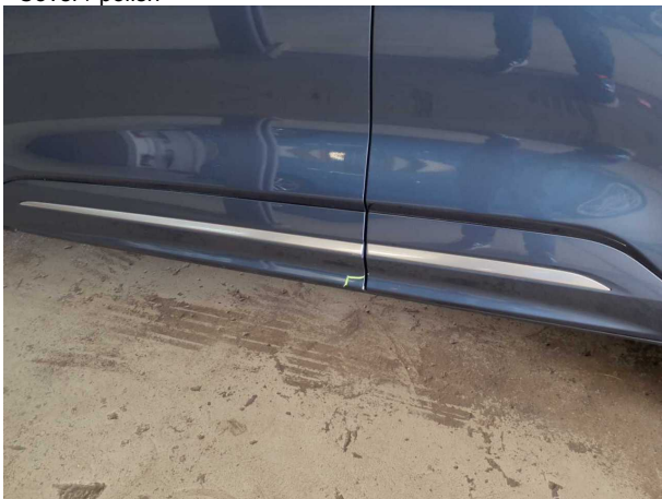
Damage #2: Door - front left side: Brightware - lower - Scratched - Smart repair
