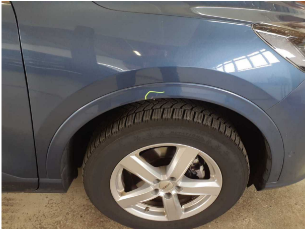
Damage #1: Mudguard - right side: Wheel well extension - Abrasi... - Cover / polish
