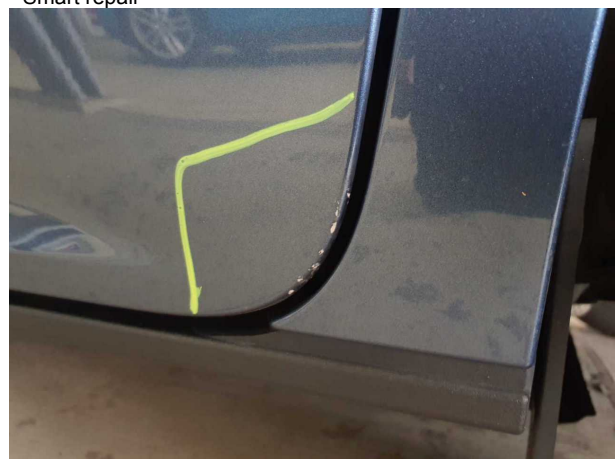
Damage #6: Door - rear left side: Brightware - lower - Scratched - Smart repair
