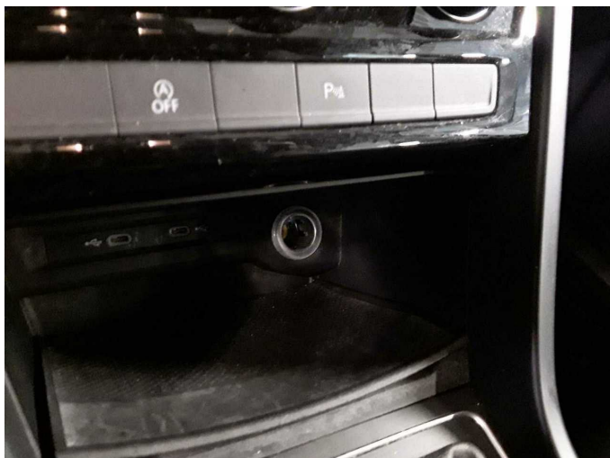
Missing part 1: Interior: Cigarette lighter - Missing - Replace
