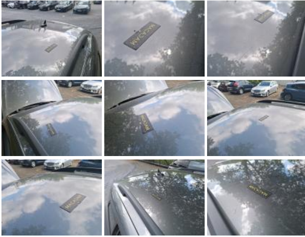
Roof, Scratch(es), Acceptable
